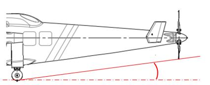
Some spacing between propeller and ground
