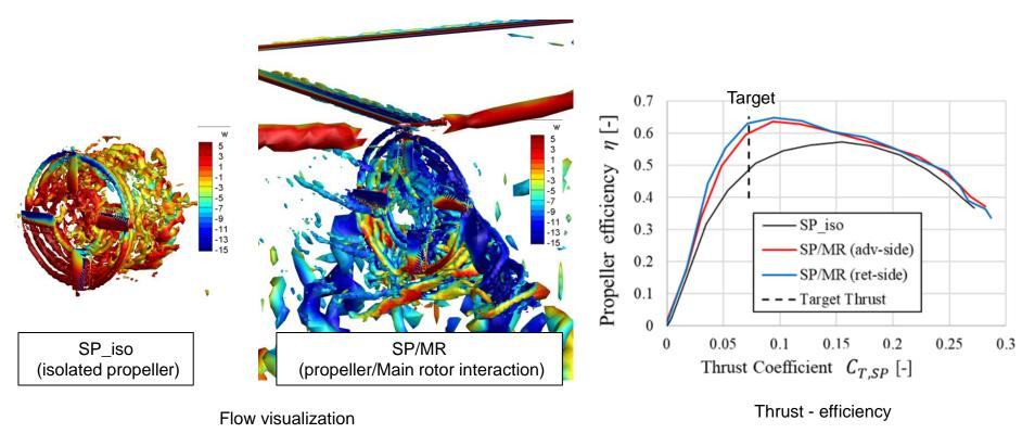
✓ CFD analysis under isolated propeller (SP\_iso) and interference condition (SP/MR)
